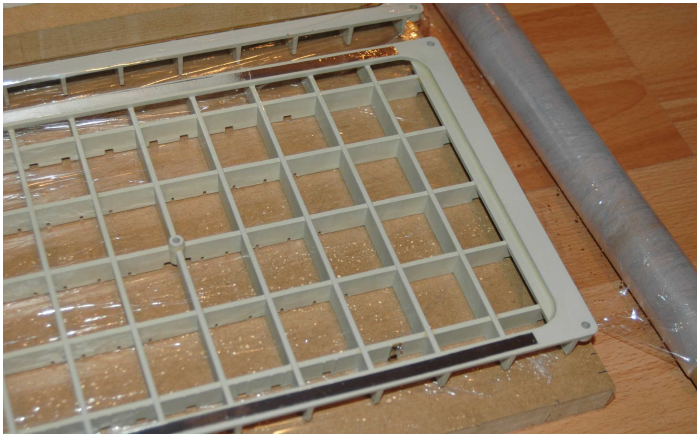
Matrix panel, as clean as a whistle, ready to receive the stator plate. The glue is barely visible. I have not used the roller(s). Instead I have used a small, strong brush to give the matrix a very thin coat of the brownish urethane glue.
